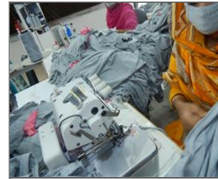
Photo of non-conformity Eye guard not using.JPG
